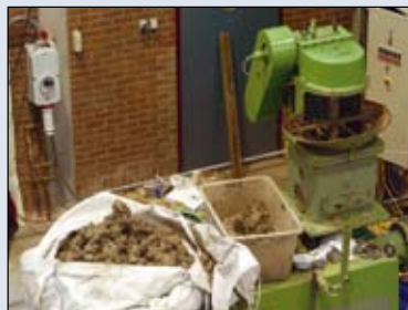
The test rig has found a temporary home at the Stevin I Laboratory of the Civil Engineering subfaculty. The semi-dried sludge from Urk harbour is delivered in big bags. An extruder then squeezes it into the installation like a big sausage.
