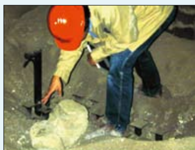
During the combustion process at 850 °C the sand and the sticky ashes can start to form lumps. This can become so serious that the whole plant has to be shut down to be cleaned by hand. The air injectors can be seen near the feet of the engineer in the picture.
