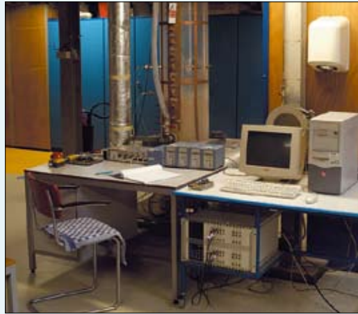
2D test bed for studying the bubble pattern in a fluidised bed for correlation with pressure fluctuations.
