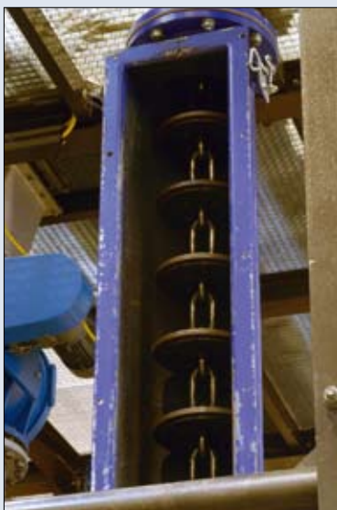
On the left the sludge sausage is pushed into the elevator where a chain fitted with discs takes over the transport. In the diagonally suspended steam vessel the balls are heated up to approximately 120 °C under a pressure of 2 bar. At the lower end of the vessel the balls pass through a lock to be added to the sludge in the elevator.
