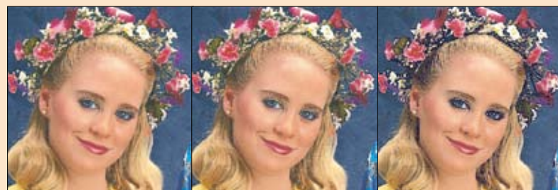
A demonstration of the method outlined in the previous figure. On the left is the original, slightly blurred image. In the centre is the result of traditional sharpening to a level that remains within the gamut. On the right is the result of the new method, which uses adaptive reduction of chromaticity to achieve even higher levels of sharpness (look at the eyes and the corner of the mouth).
